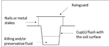
Figure 1. Cross section of a basic pitfall trap used to collect ground beetles.
