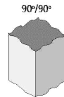
(2 cleavages, 4 faces of many possible angles; third side fractures irregularly; e.g. pyroxene, amphibole, feldspar)
