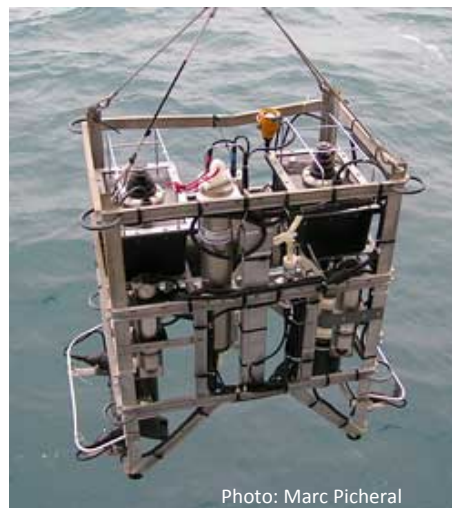
Figure 6.2. The Underwater Video Profiler and its mounted equipment
