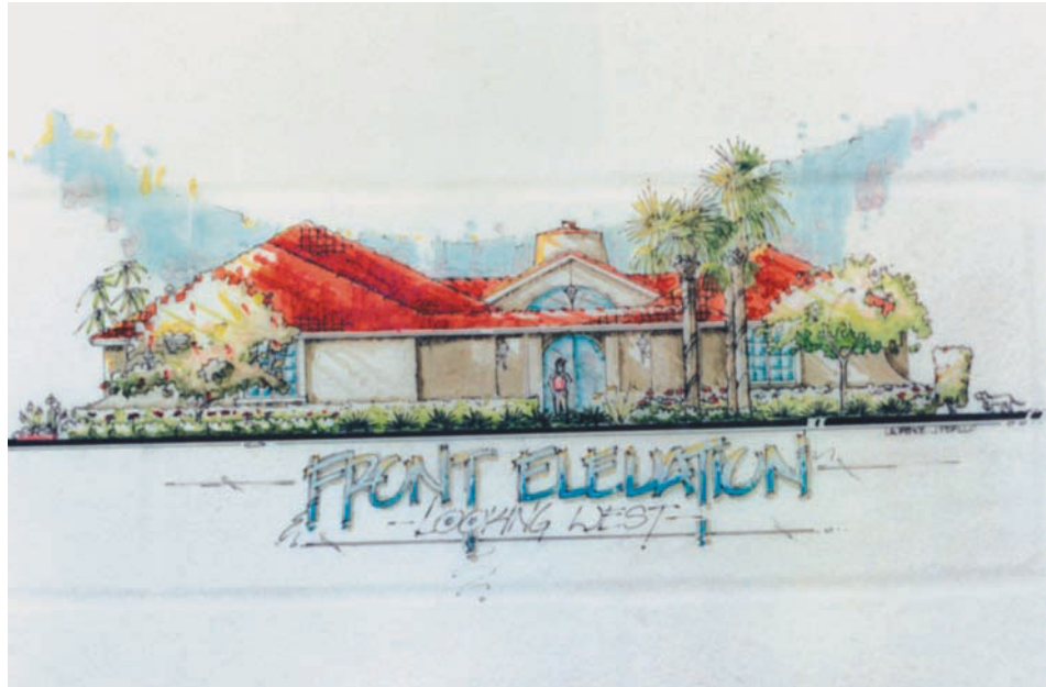
FIGURE 9–35. An elevation view permits the height and width to be drawn to scale. (Delmar/Cengage Learning)
