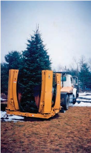
FIGURE 10-2. Large trees can be moved successfully with powered transplanters. There is limited disturbance to the root system. (Courtesy of Randy Counterline)
