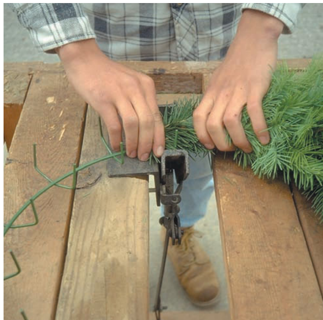
FIGURE 7–23. A wreath machine frees both hands to collect and hold the evergreen boughs in place while the foot powers the machine that wires the boughs and secures them. ( Delmar/Cengage Learning. Photo by Carroll Shry. )
