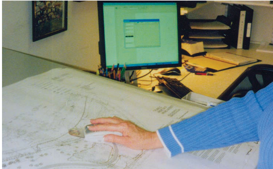
FIGURE 26-1. A hand-held stylus is used to select commands and symbols on a digitizer or menu tablet. (Delmar/Cengage Learning. Photo by Jack Ingels.)
