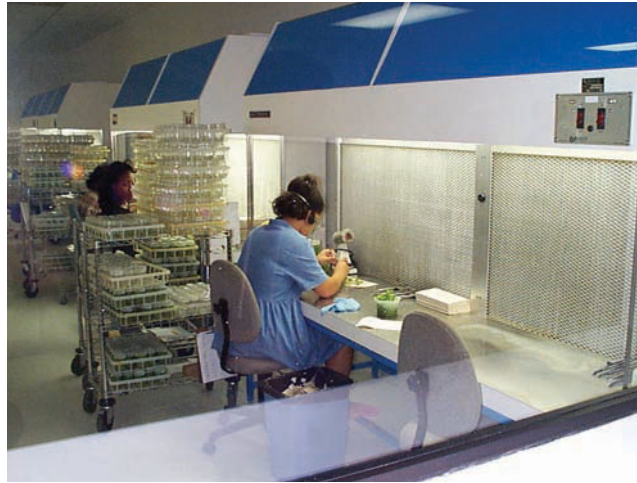
FIGURE 14–19. A transfer chamber requires an antiseptic environment, a heat source to flame instruments prior to each use, and a supply of sterilized media and containers. ( Delmar/Cengage Learning )
