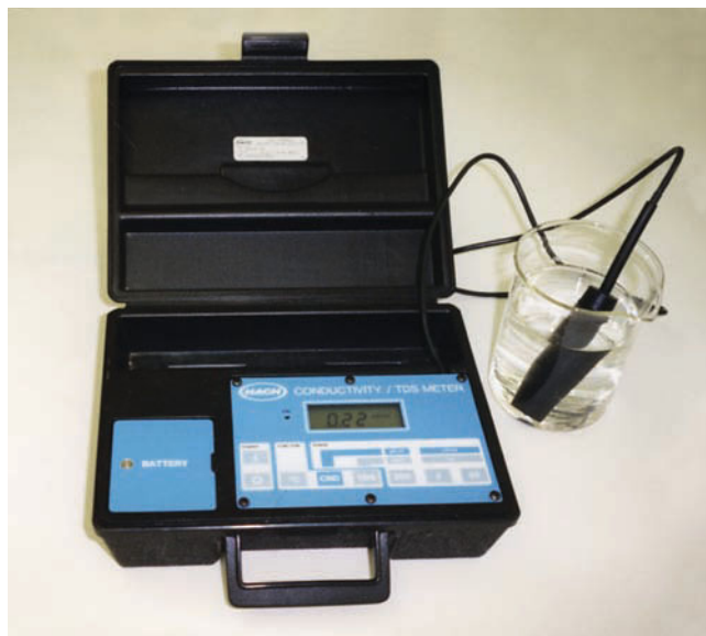
FIGURE 20–3. A conductivity/TDS meter is used to test the total soluble salt levels of solutions and media. (Delmar/Cengage Learning. Photo by Jack Ingels.)
