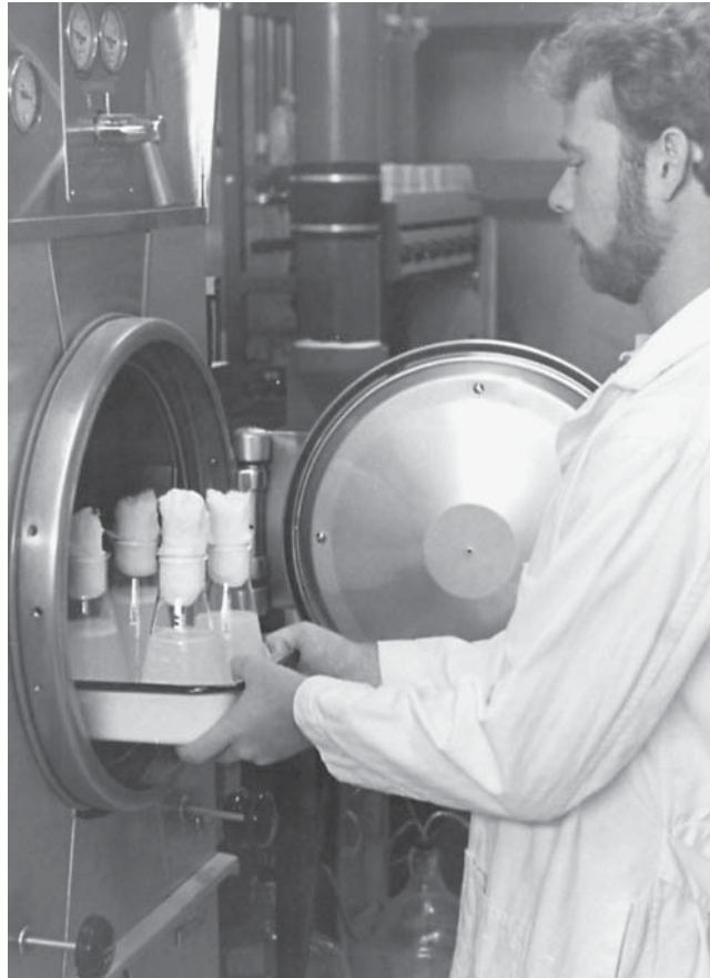
FIGURE 14–20. A laboratory autoclave provides steam heat under pressure to sterilize media, tools, and containers. Here flasks of agar are being set into the autoclave. ( Delmar/Cengage Learning )
