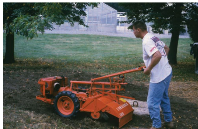
FIGURE 13-9. A rototiller is an excellent way to incorporate additives into the soil while loosening it. (Delmar/Cengage Learning. Photo by Jack Ingels.)
