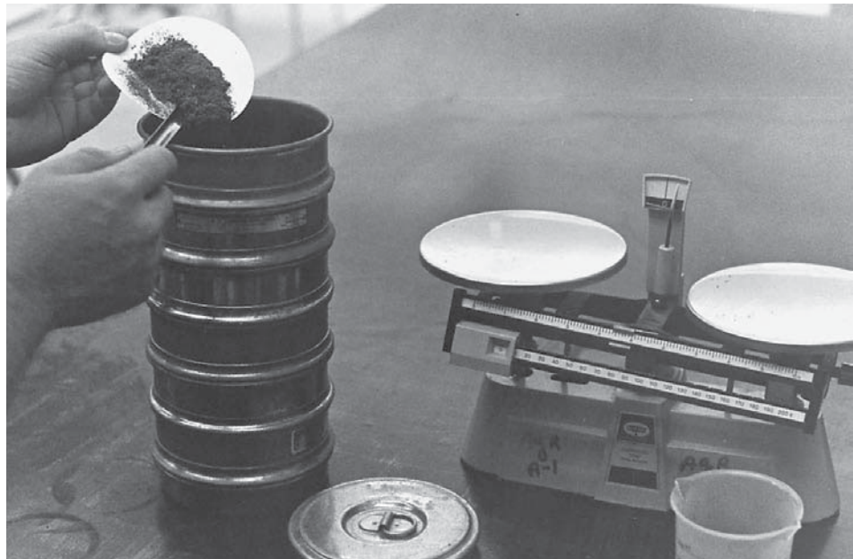
FIGURE 3–2. To use soil sieves, a premeasured amount of dried soil is passed through the stack. Each sieve's mesh is finer than the one before. Sands are separated by particle size. An additional suspension and setting technique is required to measure the percentage of silt and clay. (Delmar/Cengage Learning. Photo by Jack Ingels)
