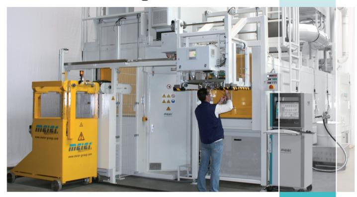
Our hot impregnation systems in the resistance heating sector are based on the principle of low frequency heating - a decisive advance over normal systems using direct current heating.
