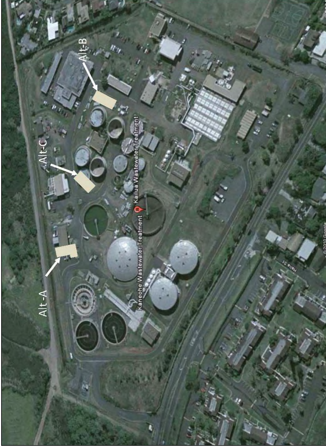
Figure 34. Alternative locations for the new dewatering building at the Kailua WWTP (source: Google 2010, provided by client)
