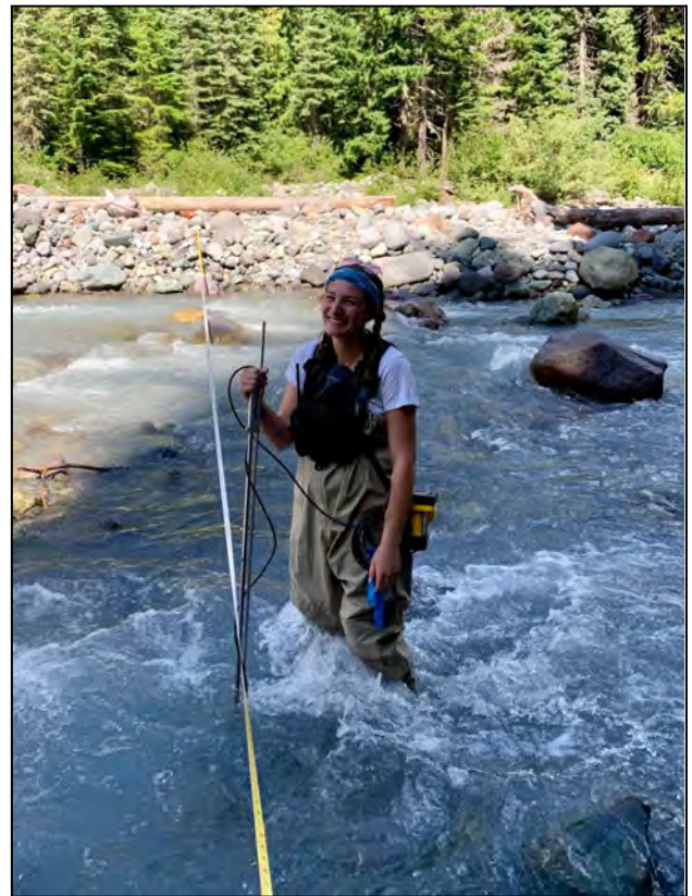
Rachel Fricke measuring discharge on the White River in Mt. Rainier National Park Photo: Rachel Fricke
