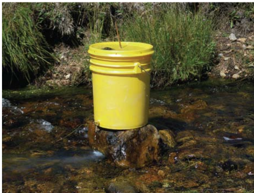
A rotenone drip station used by New Mexico Department of Game and Fish on Costilla Creek in September 2008. CFT legumine (5% rotenone) was applied at a constant rate for four hours to obtain an initial concentration of 50 ppb active rotenone. The project was part of a Rio Grande cutthroat trout ( Oncorhynchus clarki virginalis ) restoration project.
