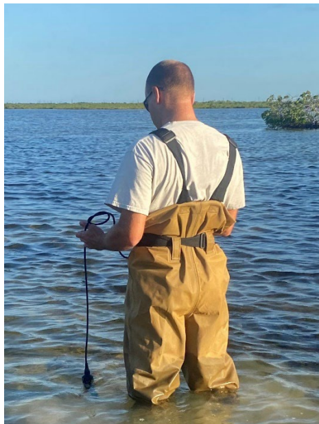
Florida Keys Aquatic Preserve staff conducting field water quality sampling using a YSI ProDSS Water Quality Meter.
