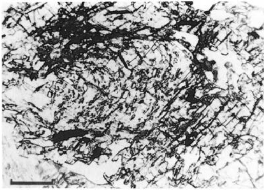
Fig. 10. Garnet from micaschist of the Nordåsvatn Complex, MiBA, showing an inner core with fine-grained inclusions defining a curved foliation, and an outer rim with more randomly oriented, coarser inclusions. Locality 4. Scale bar: 1 mm.
