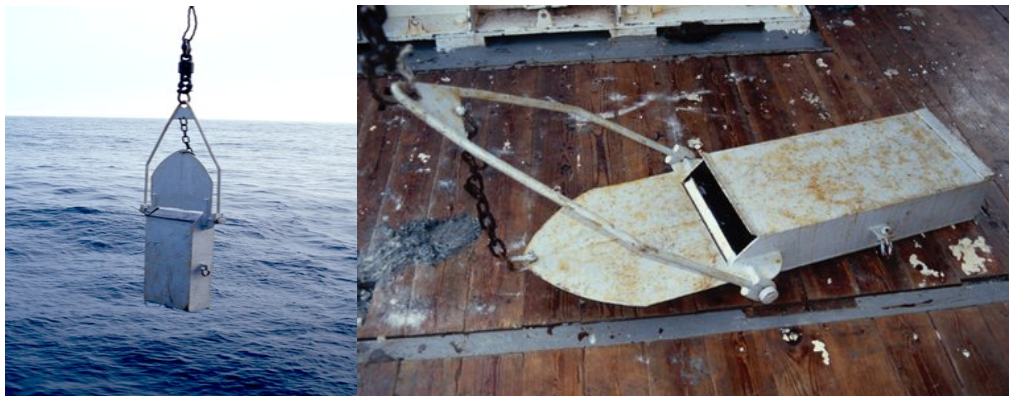
Figure 25: Anchor dredge before being lowered to the seafloor and on deck of R/V Tangaroa .
