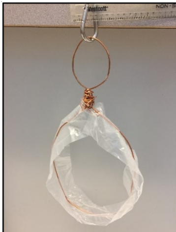
Figure 9.1. LDPE sampler for water column.
