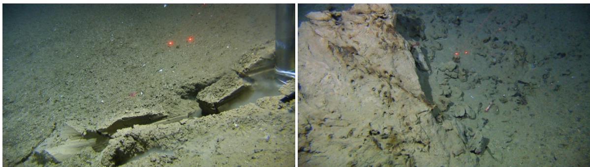
Seabed types at 2000 m water depth. Picture on the left shows foot of video-rig sinking into soft mud. Picture on the right shows compacted sediment block with gravel. Ten centimeters between red laser points.
