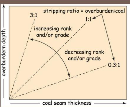
Surface vs. Underground Mining: Cutoff Depth
