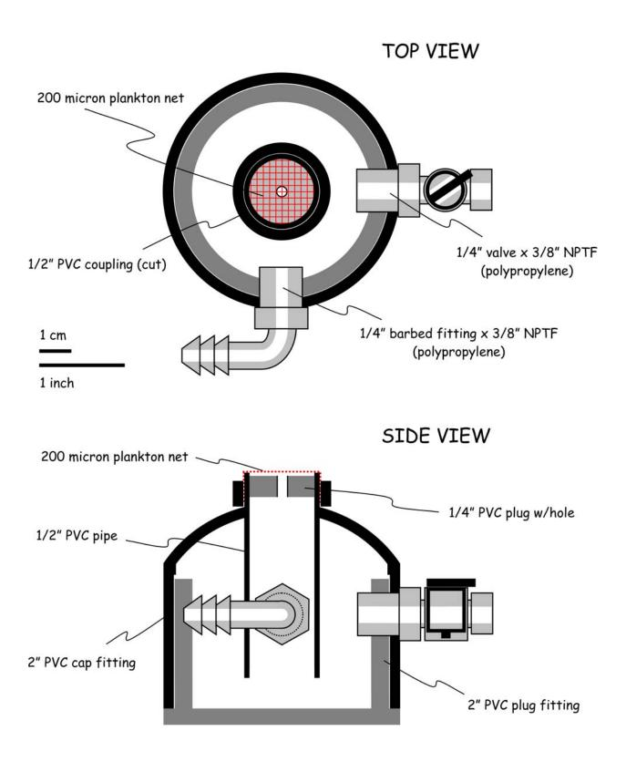
Figure 3.1. Schematic representation of the dewatering device used for the non-disruptive, vacuum-assisted, removal of water (external medium) from live acoels prior to weighing the animals. The device was fabricated from common PVC pipe and fittings.
