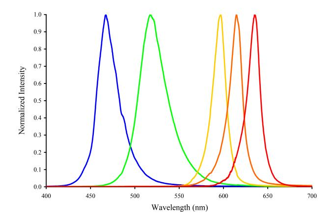
Figure 4.5. Normalized output spectra of the five light emitting diodes used in the photophobic response experiments. Wavelength peaks were at 470, 525, 589, 610, and 630 nm respectively for the blue, green, yellow, orange, and red LED lamps.
