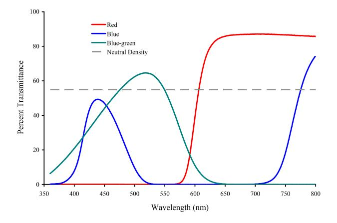
Figure 4.3. Transmittance spectra of the filters used in determining and defining the short-term response of *Convolutriloba retrogemma* to a step-up, sudden increase in light intensity. These filters were used in conjunction with a halogen, fiber-optic light source.
