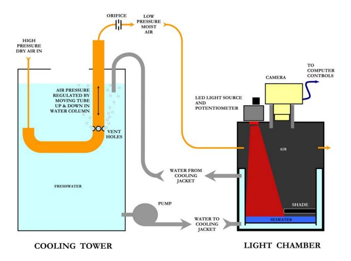
Figure 4.2. Schematic representation of light chamber and time-lapse photography apparatus utilized in the photomovement experiments. Light-source was interchangeable. Experiments used either a halogen/fiberoptic light-source with optical filters or monochromatic, light emitting diode arrays (shown).
