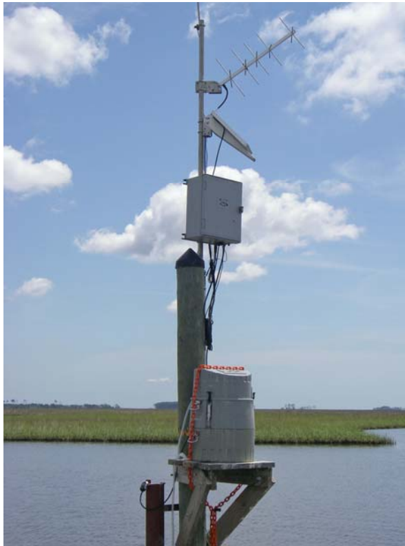
ISCO water sampler and telemetered data sonde in Bangs Lake. Photo credit: Christine Walters.
