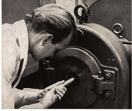
Swaging machine forms aluminum barrel jacket over stainless steel liner in fast operation for low-cost construction of erosion-resistant AR-10 barrels.
