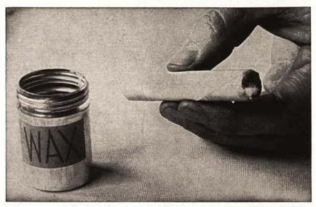
Tube was covered with outer wrap of stiff paper, powder poured in, and bullet inserted. Bullet end was crimped and dipped in hot lubricant of tallow and wax.
