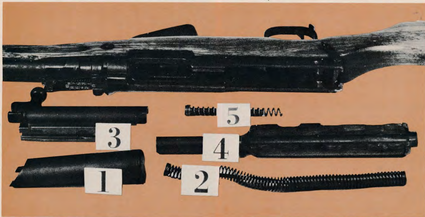
The parts of the SKS as they are removed for cleaning: 1. Receiver cover; 2. Captive recoil spring assembly; 3. Bolt and bolt carrier assembly; 4. Upper handguard assembly housing the gas cylinder tube; 5. Gas piston and spring. Receiver cover, operating handle and bolt are stamped with serial numbers. This action is basically a scaled-down version of the obsolete PTRS antitank rifle system.
