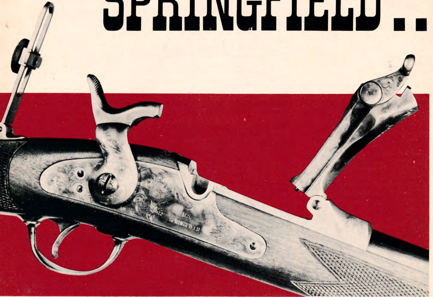
The classic Trapdoor action, shown open at top for loading. Bottom photo shows receiver and tang in one piece; original '73's had these as separate units. Color photo of the Officer's Model on facing page courtesy of Harrington & Richardson, Inc.
