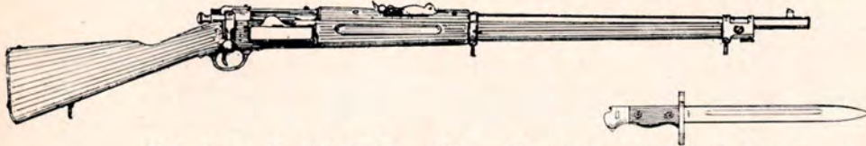
U.S. Krag Model 1898, caliber .30-40, five-shot bolt action.
