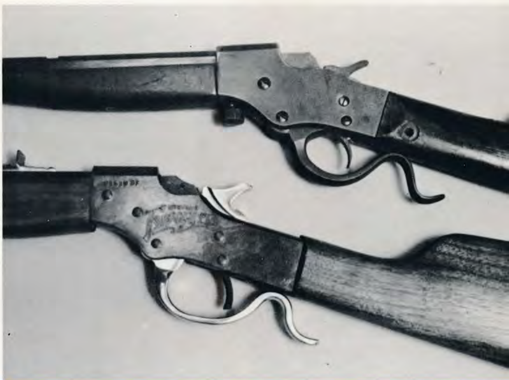
Side view illustrates the larger finger-lever and omission of the take-down screw at the bottom, front of the receiver. Also, the new Favorite's hammer and finger-lever are plated. Receiver is color case-hardened with a gold inscription on both sides.
