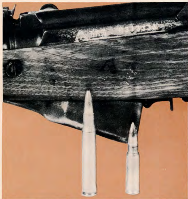
Soviet 7.62mm Model 1943 cartridge (right) appears to be a refinement of the 7.92mm Kurz developed by the Germans during World War II. A .30-06 is shown at left. Note lengthy serial number on the receiver.
