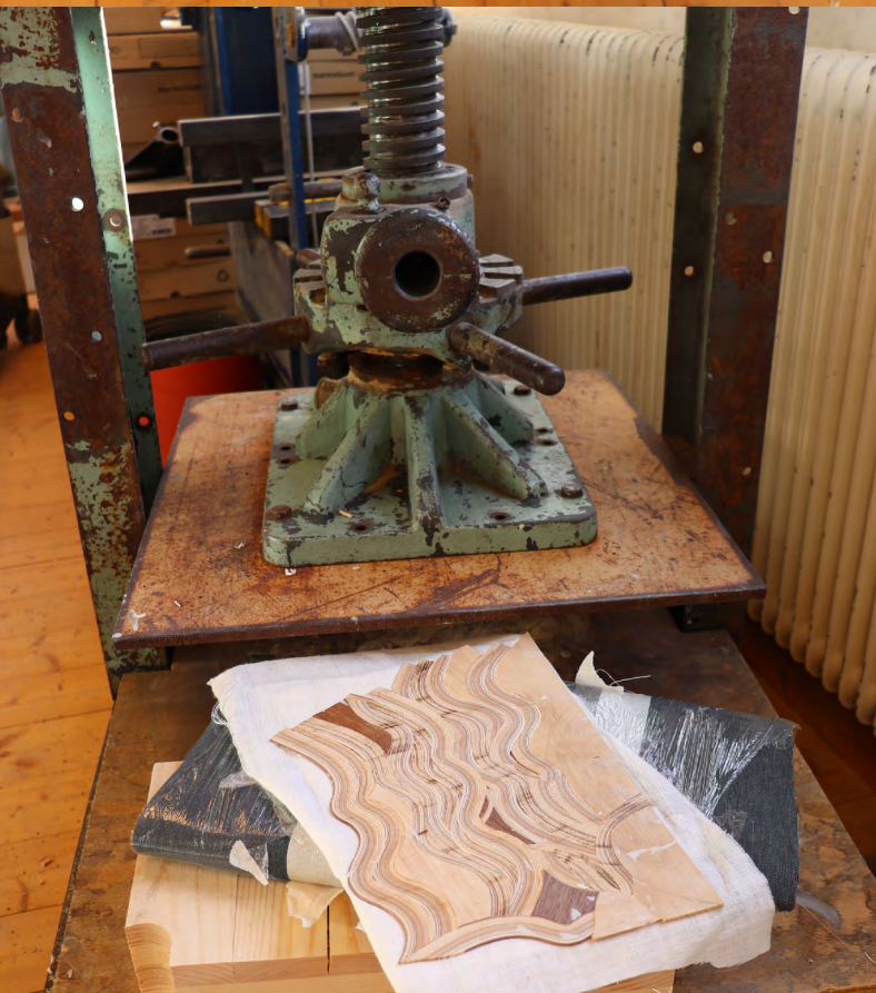
Figure 30. Making of 'Flammes' marquetry surface with the scroll saw before pressing and gluing it flat with the hand press (2021).
