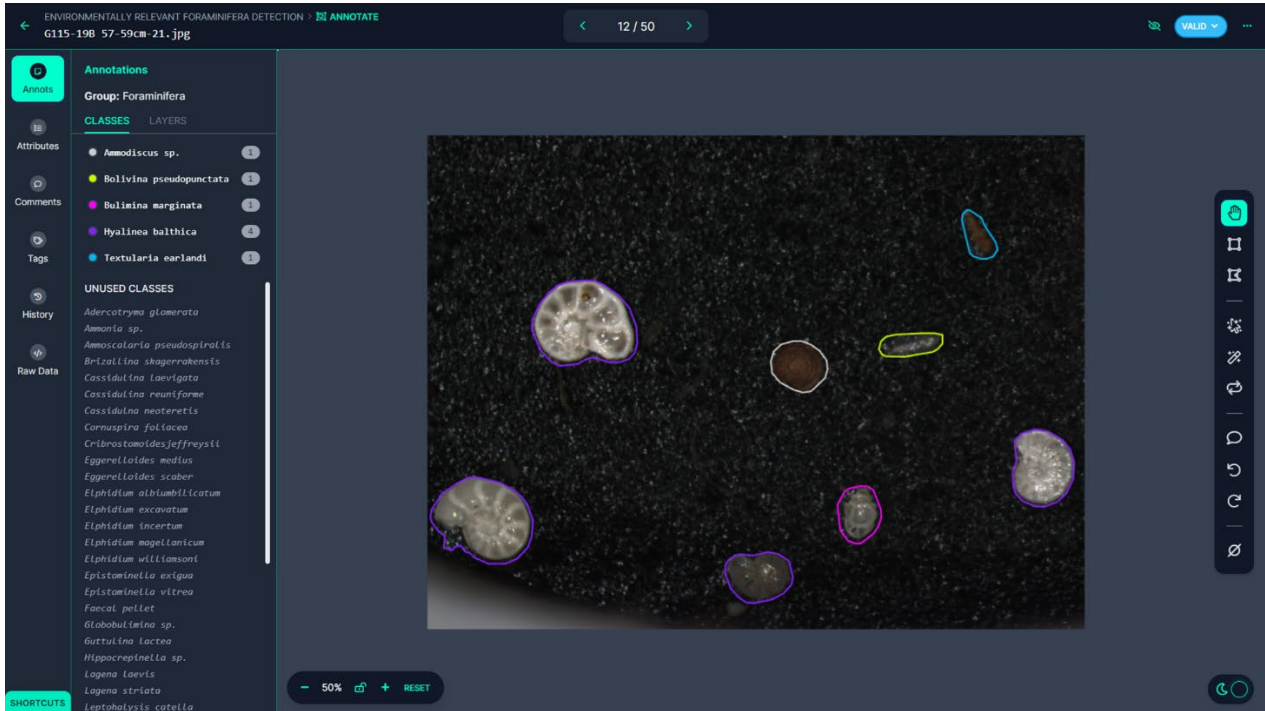
Figure 6. Roboflow interface for classifying individual foraminifera in an image. On the left side of the window, there is a color-coded list of labelled foraminifera in an image on the right. On the rightmost side, there is a tool selection panel, from which a user can label foraminifera either by using an automatic feature extraction tool or by manually drawing a polygon around the foraminifera.
