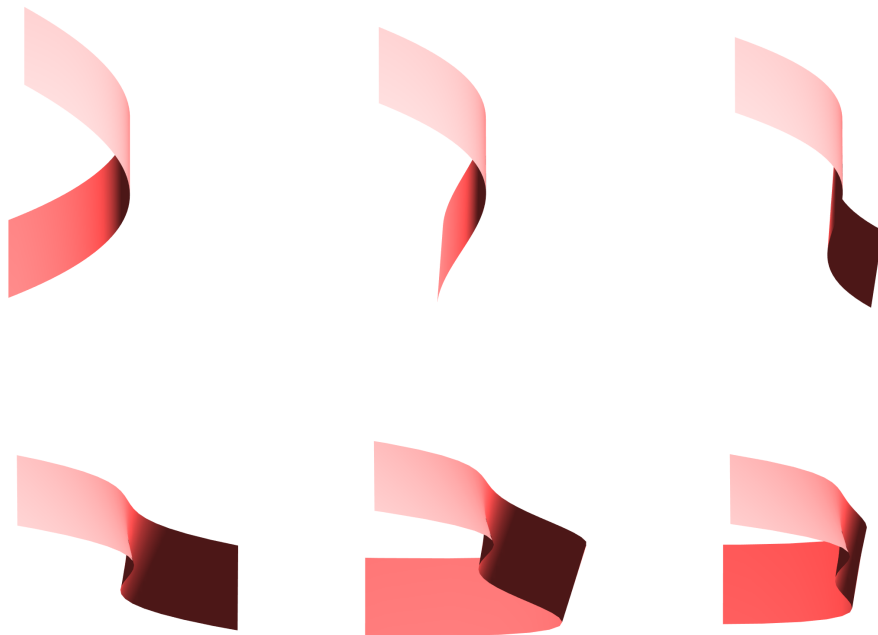
Figure 34: Evolution of Thom's elementary catastrophes with potential V_\tau = (1 - \tau)V_1 + \tau V_2 from the V_{fold} (first frame) to the V_{cusp} (4th frame) and to the V_{swallowtail} (last frame). The equilibrium manifold \frac{\partial V(x,p)}{\partial x} = 0 is visualised.
