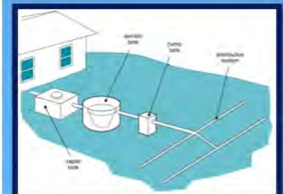
Figure 2. ATU in septic system.
