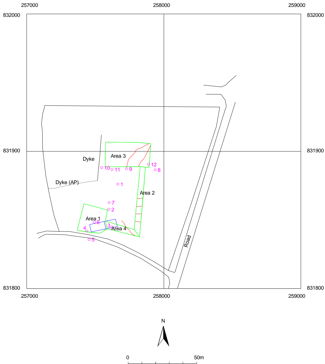
Figure 2 Plan of site showing area of topsoil strip (green); existing building (blue) and land drains (red)
