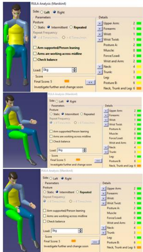
Figure 30: Nigerian Male Manikin 95 th percentile in Stature Postured as a Third Row Passenger in the Vehicle Package using 340mm as the Seat Height (H30) Value with Right, Center and Left Seating Positions (top, middle and bottom images respectively)
