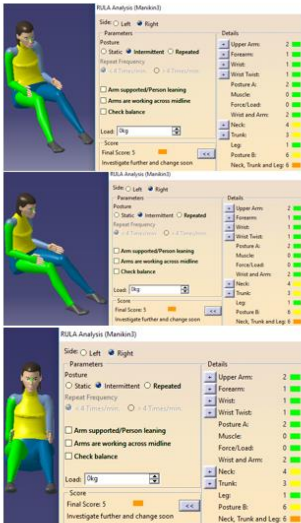
Figure 29: Nigerian Female Manikin 5 th percentile in Stature Postured as a Third Row Passenger in the Vehicle Package using 340mm as the Seat Height (H30) Value with Right, Center and Left Seating Positions (top, middle and bottom images respectively)
