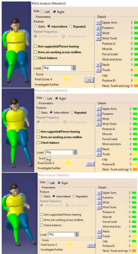
Figure 33: Nigerian Female Manikin 5 th percentile in Weight Postured as a Second Row Passenger in the Vehicle Package Based on SAE J1100 Package Dimensions with Right, Center and Left Seating Positions (top, middle and bottom images respectively)
