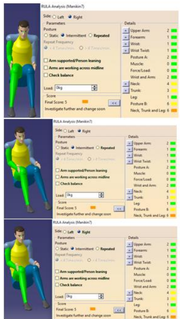
Figure 44: Nigerian Male Manikin 95 th percentile in Sitting Height Postured as a Second Row Passenger in the Vehicle Package Based on SAE J1100 Package Dimensions with Right, Center and Left Seating Positions (top, middle and bottom images respectively)
