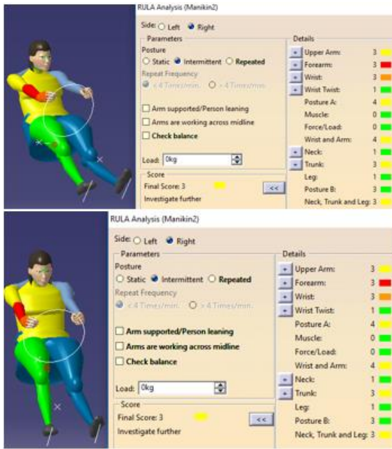
Figure 14: Nigerian Female Manikin 5 th percentile in Weight Postured as a Driver in the Vehicle Package using 340mm as the Seat Height (H30) Value with Automatic and Manual Transmission Selection (top and bottom images respectively)
