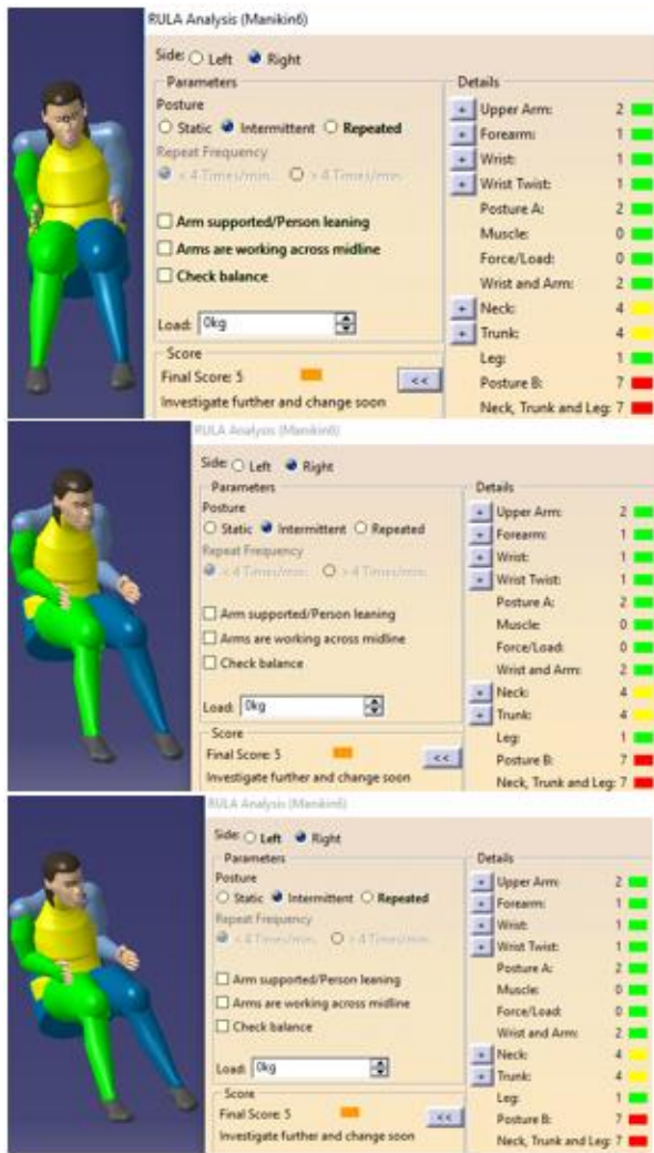
Figure 45: Nigerian Female Manikin 5 th percentile in Sitting Height Postured as Second Row Passenger in the Vehicle Package using 340mm as the Seat Height (H30) Value with Right, Center and Left Seating Positions (top, middle and bottom images respectively)
