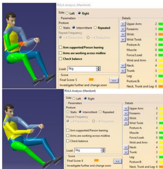
Figure 11 Nigerian Male Manikin 95 th percentile in Stature Postured as a Driver in the Vehicle Package Based on SAE J1100 Package Dimensions with Automatic and Manual Transmission Selection (top and bottom images respectively)
