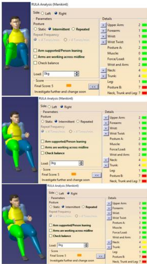
Figure 49: Nigerian Female Manikin 5 th percentile in Sitting Height Postured as a Third Row Passenger in the Vehicle Package using 340mm as the Seat Height (H30) Value with Right, Center and Left Seating Positions (top, middle and bottom images respectively)
