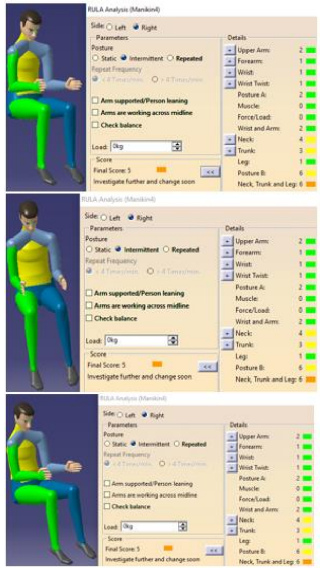
Figure 28: Nigerian Male Manikin 95 th percentile in Stature Postured as a Third Row Passenger in the Vehicle Package Based on SAE J1100 Package Dimensions with Right, Center and Left Seating Positions (top, middle and bottom images respectively)
