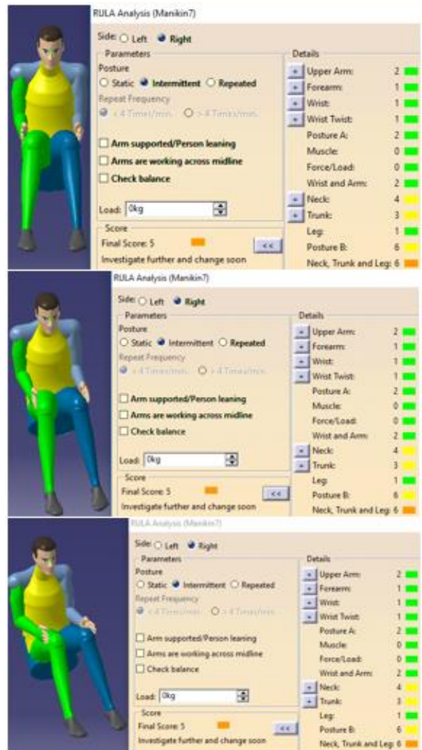
Figure 46: Nigerian Male Manikin 95 th percentile in Sitting Height Postured as a Second Row Passenger in the Vehicle Package using 340mm as the Seat Height (H30) Value with Right, Center and Left Seating Positions (top, middle and bottom images respectively)
