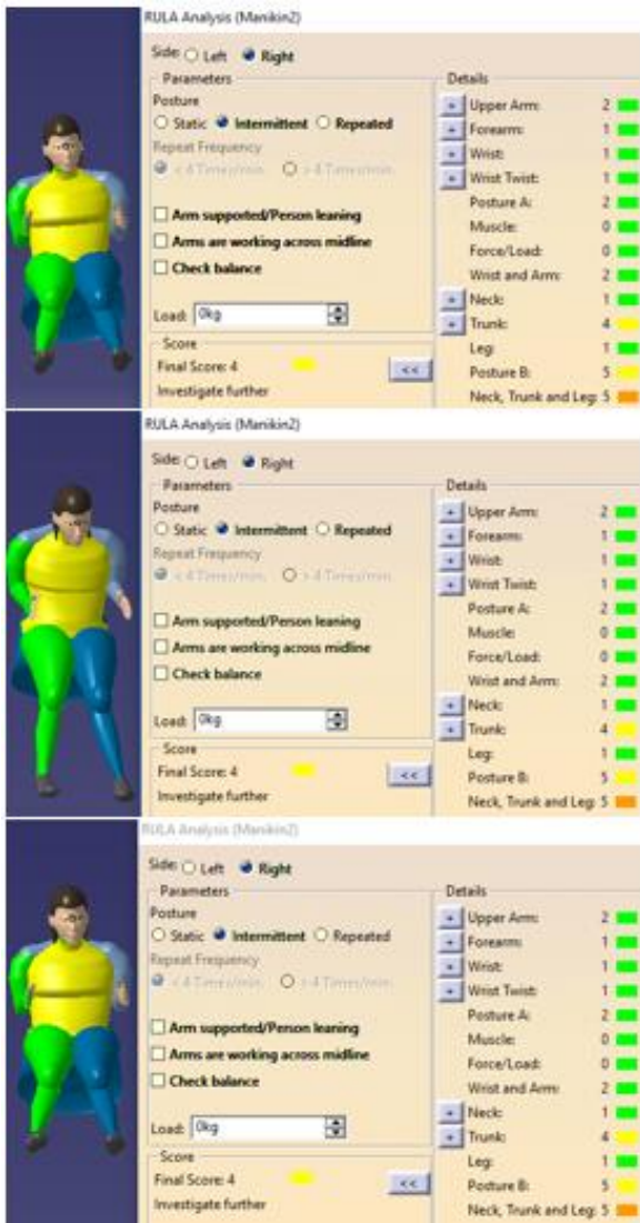
Figure 37: Nigerian Female Manikin 5 th percentile in Weight Postured as a Third Row Passenger in the Vehicle Package Based on SAE J1100 Package Dimensions with Right, Center and Left Seating Positions (top, middle and bottom images respectively)
