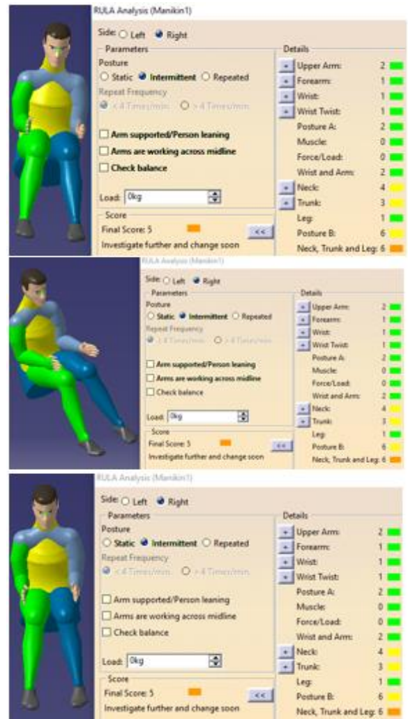
Figure 34: Nigerian Male Manikin 95 th percentile in Weight Postured as a Second Row Passenger in the Vehicle Package Based on SAE J1100 Package Dimensions with Right, Center and Left Seating Positions (top, middle and bottom images respectively)
