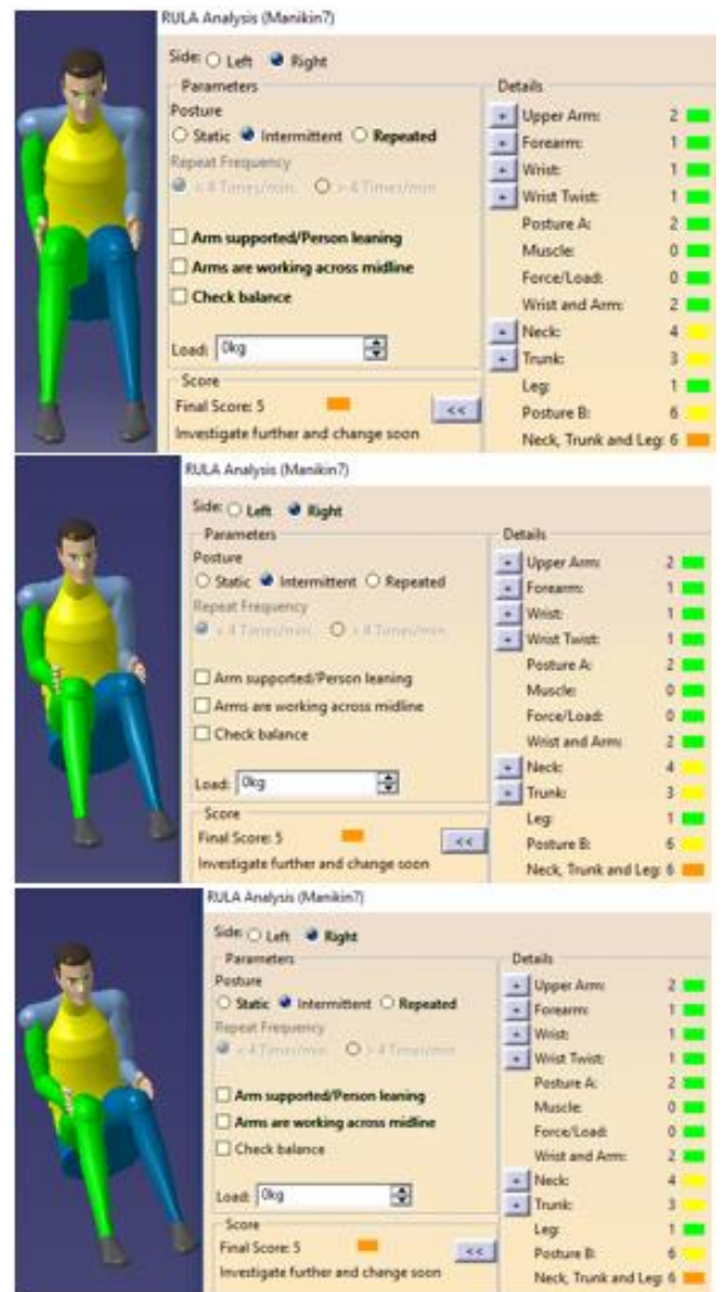
Figure 48: Nigerian Male Manikin 95 th percentile in Sitting Height Postured as a Third Row Passenger in the Vehicle Package Based on SAE J1100 Package Dimensions with Right, Center and Left Seating Positions (top, middle and bottom images respectively)
