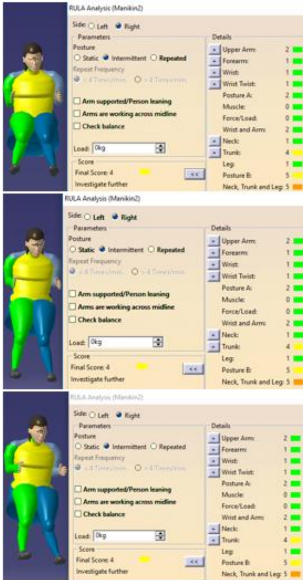
Figure 39: Nigerian Female Manikin 5 th percentile in Weight Postured as a Third Row Passenger in the Vehicle Package using 340mm as the Seat Height (H30) Value with 340mm as the Seat Height (H30) Value with Right, Center and Left Seating Positions (top, middle and bottom images respectively)
