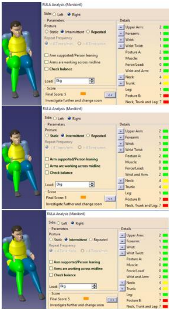
Figure 43: Nigerian Female Manikin 5 th percentile in Sitting Height Postured as Second Row Passenger in the Vehicle Package Based on SAE J1100 Package Dimensions with Right, Center and Left Seating Positions (top, middle and bottom images respectively)
