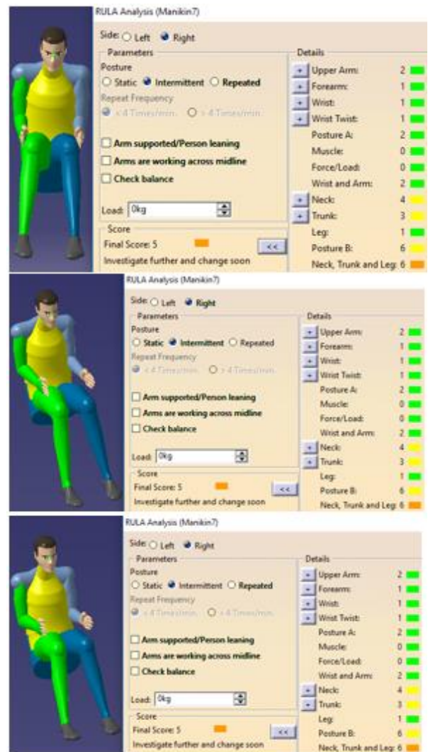
Figure 50: Nigerian Male Manikin 95 th percentile in Sitting Height Postured as a Third Row Passenger in the Vehicle Package using 340mm as the Seat Height (H30) Value with Right, Center and Left Seating Positions (top, middle and bottom images respectively)
