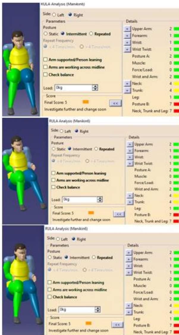
Figure 47: Nigerian Female Manikin 5 th percentile in Sitting Height Postured as a Third Row Passenger in the Vehicle Package Based on SAE J1100 Package Dimensions with Right, Center and Left Seating Positions (top, middle and bottom images respectively)
