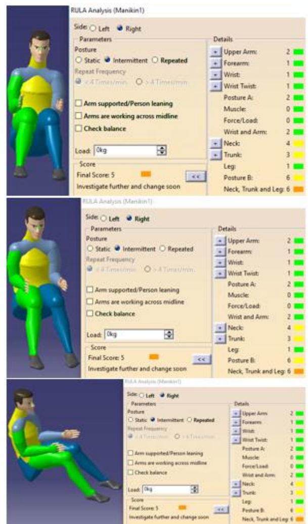
Figure 36: Nigerian Male Manikin 95 th percentile in Weight Postured as a Second Row Passenger in the Vehicle Package using 340mm as the Seat Height (H30) Value with Right, Center and Left Seating Positions (top, middle and bottom images respectively)
