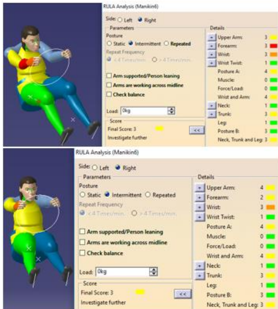
Figure 17: Nigerian Female Manikin 5 th percentile in Sitting Height Postured as a Driver in the Vehicle Package Based on SAE J1100 Package Dimensions with Automatic and Manual Transmission Selection (top and bottom images respectively)
