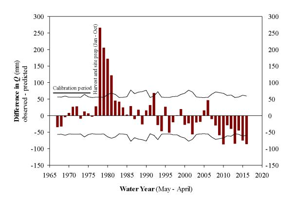
Discharge increased substantially for four years following harvest, then remained similar to the reference watershed for the next 25 years. At that time, discharge became consistently and sometimes significantly lower than in the reference watershed.
