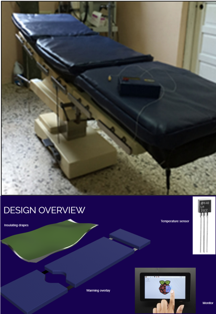
The prototype and design overview of the PeriOperative team's automated surgical warming mattress.
