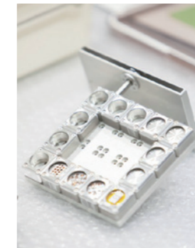
↑ Example of ExHAM experimental samples. The samples are arranged inside the 10-cm square adapter. → Small satellite launched from the JEM Small Satellite Orbital Deployer (J-SSOD)
