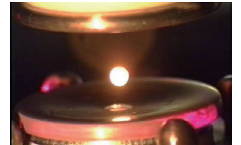
A high-temperature sample floating in the Electrostatic Levitation Furnace on Earth. In space, results are expected for materials that are more difficult to electrically charge.
