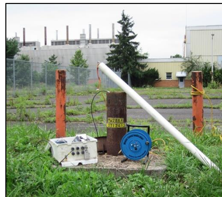
Figure 1. Slug testing setup at a monitoring well.
