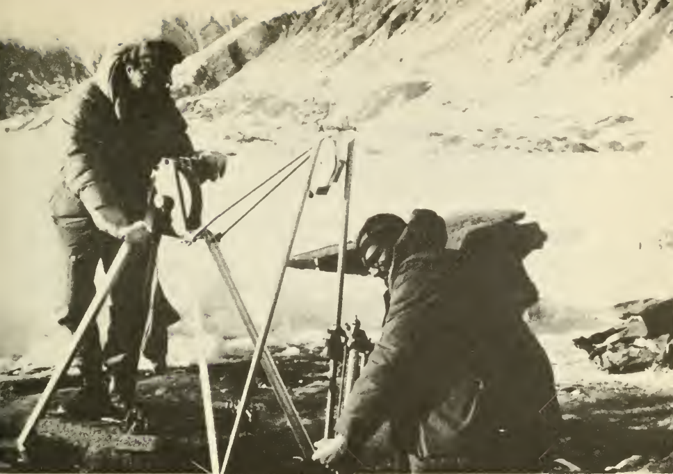
James E. Mielke (left) and Austin Long collecting water samples at Tuborg Lake on Ellesmere Island. Knudsen bottles are lowered with the hand winch through an 8-inch-diameter hole in the ice to the sampling depth, a messenger dropped along the line closes the bottle, and the sample is drawn up. At least 20 liters are collected from each depth.
