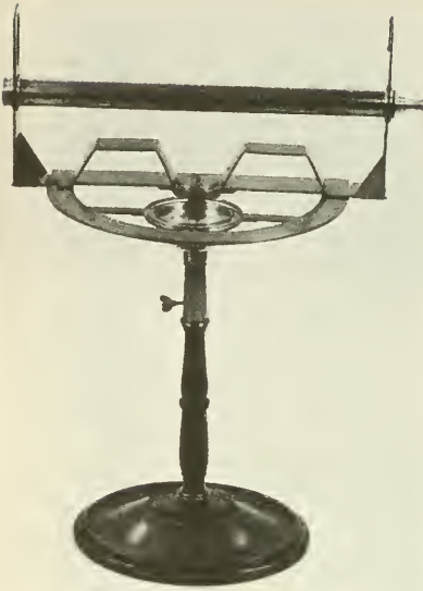
Eighteenth-century semicircumferentor by Pavolini, showing an early use of a telescopic sight on a surveying instrument.
