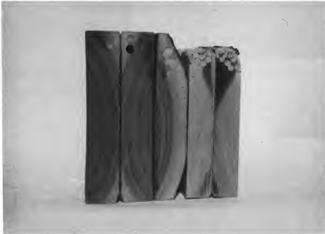
Figure 1. Black polycaon damage to hardwood taken from a lumber yard in Santa Ana, California.
