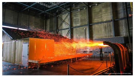
Figure 10. Testing deck vulnerability to embers at the IBHS Research Center. IBHS and others have <u>conducted extensive testing</u> regarding the vulnerability of decks<sup>53</sup> and fences.<sup>54</sup>
