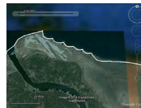
Rosetta sea wall and sea groins. The groins reduced erosion locally, the problem is transferred eastward. From left to right: 2003, 2009, 2016. The white line corresponds to the 2009 coastline.
