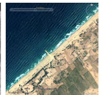
Arish port. Coastal groins eastward to stop erosion. Erosion issues transferred eastward of the groin system.
