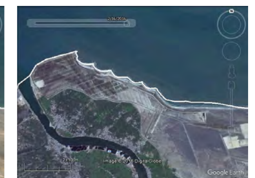
Rosetta sea wall and sea groins. The groins reduced erosion locally, the problem is transferred eastward. From left to right: 2003, 2009, 2016. The white line corresponds to the 2009 coastline.
