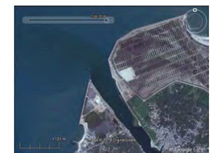
Rosetta sea wall and sea groins. The groins reduced erosion locally, the problem is transferred eastward. From left to right: 2003, 2009, 2016. The white line corresponds to the 2009 coastline.
