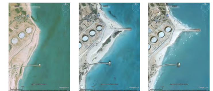
El Hamra Petroleum Port. Building of the sea groins in a highly dynamical environment. Erosion and saltation issues
