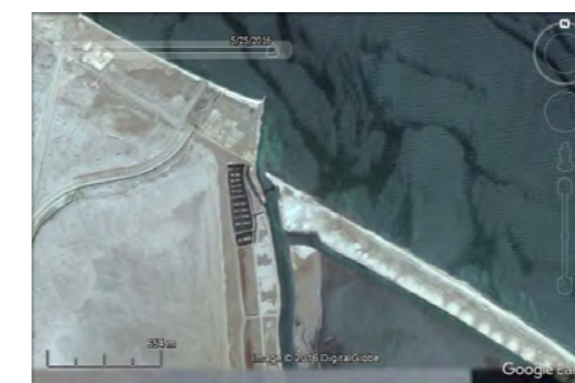
Sahl El Tina western drain (west of Port Said port) and internal wall of the sand barrier. Siltation issues. Top: 2011, bottom: 2016.
