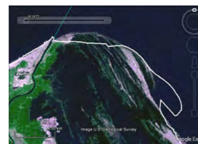
Morphological evolution of Damietta ridges. From left to right: 1978, 2010, 2016. The white line corresponds to the 2010 coastline. The northern part is rigid (Damietta E wall), erosion eastward.
