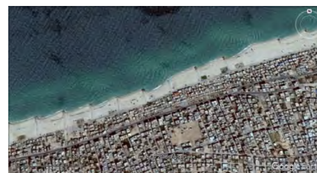
The Arish beach sea groin system protruding in a very active surf zone. The initial (2009 image) structures do not impede erosion and have been extended (2011 image). The problem is partially (locally) solved, it is transferred eastward.
