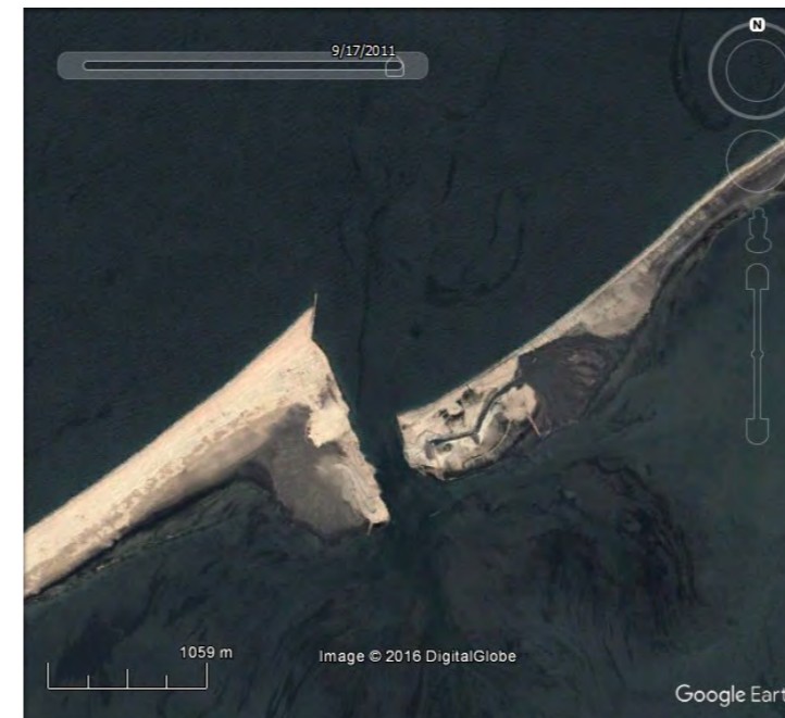
Bardawil western inlet. Sand deposition westward and sand deficit eastward. The sea groin broke the continuity of the sand barrier and impede the free behavior of the system.
