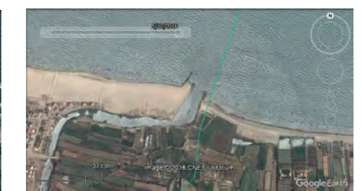
Eastern sea groins of Baltim and Kitchener drain. Siltation issues in Kitchener drain and erosion eastward. Left: 2007, right: 2016.
