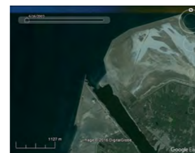
Rosetta sea wall and sea groins. The groins reduced erosion locally, the problem is transferred eastward. From left to right: 2003, 2009, 2016. The white line corresponds to the 2009 coastline.
