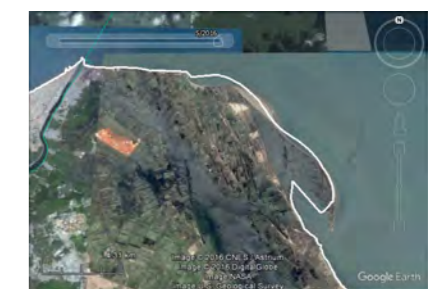
Morphological evolution of Damietta ridges. From left to right: 1978, 2010, 2016. The white line corresponds to the 2010 coastline. The northern part is rigid (Damietta E wall), erosion eastward.
