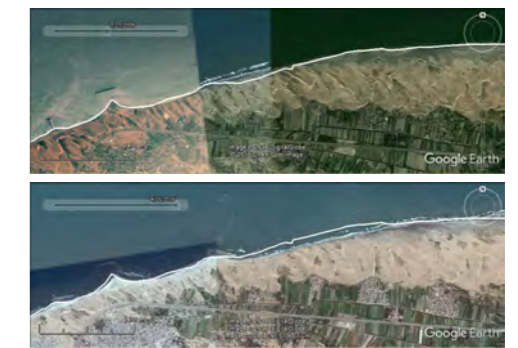
Erosion eastward the Bourg El Burullus detached breakwaters.
