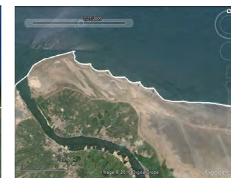
Rosetta sea wall and sea groins. The groins reduced erosion locally, the problem is transferred eastward. From left to right: 2003, 2009, 2016. The white line corresponds to the 2009 coastline.
