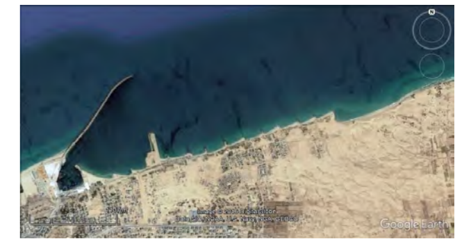
Arish port. Coastal groins eastward to stop erosion. Erosion issues transferred eastward of the groin system.
