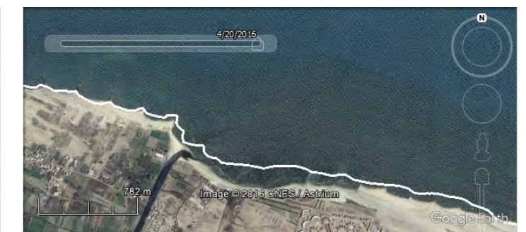
Eastern sea groins of Baltim and Kitchener drain. Siltation issues in Kitchener drain and erosion eastward. Left: 2007, right: 2016.
