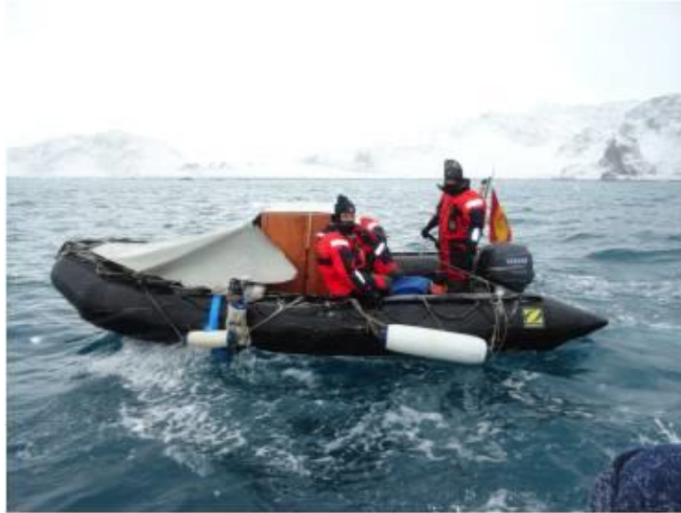
Figure 4. Very shallow water bathymetry system operated from a small rubber boat
