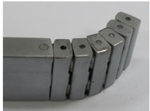
Fig. 12. The newly designed mandrel along with the assembled cores.
