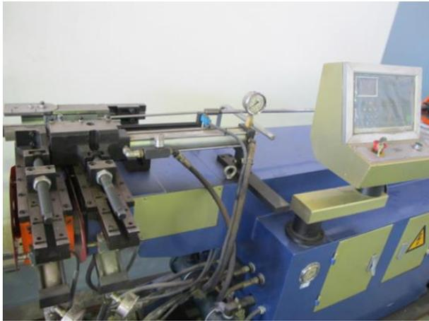
Fig. 7. NC bending machine.
