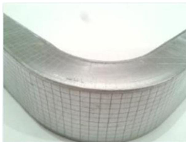
**Fig. 13.** Successful profile bending on the annealed heated rectangular cross sectional aluminum.
