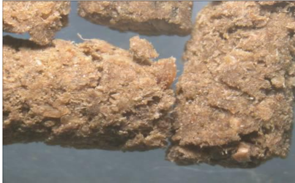
Figure 12. Poor quality pellet (20 x) (Kop et al.,2006).
