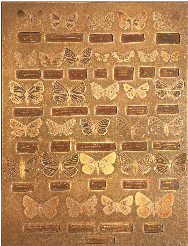
Fig. 3. Copper printing plate used to apply the color yellow for Plate 53 of Butterflies of California .
