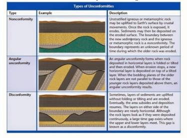
Unconformity. An unconformity is a widespread surface separating rocks above and below, which represents a gap in the rock record
