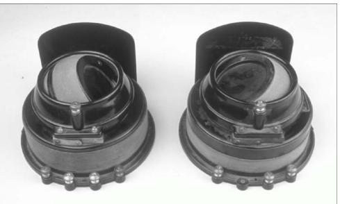
**Figure 4-10.** Coupled circuit tuners, first version (left), and second version (right).
