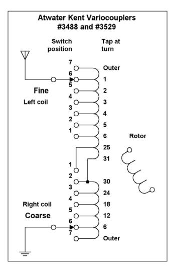
Figure 4-6. Schematic of variocoupler.
