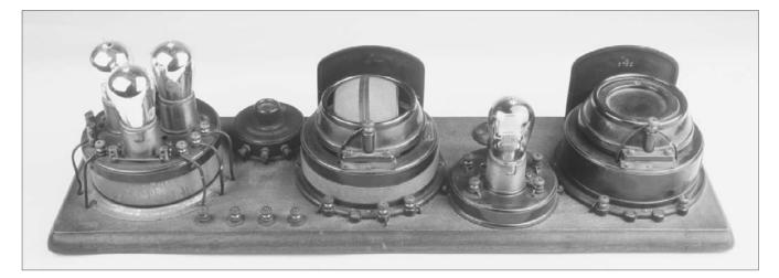
Figure 4-13. Type II tuner (right) on Model 9 # 4445 open set, rear view.
