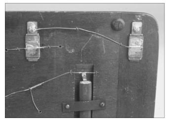
Figure 4-15. Antenna capacitors, bottom view.
