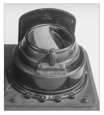
**Figure 4-14.** Type II tuner, third version, on Model 9A # 4445A, rear view.
