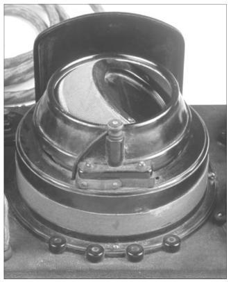
Figure 4-11. The coupled circuit tuner, third version, mounted on a Model 9A # 4445A open set, rear view.
