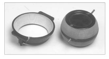
Figure 4-2. Variometer #3488 stator (left) and rotor.
