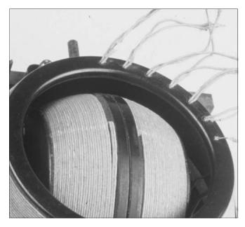
Figure 4-7. Detail of early variocoupler switch wiring and bifilar rotor.
