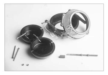
Figure 4-5. Disassembled early variocoupler.
