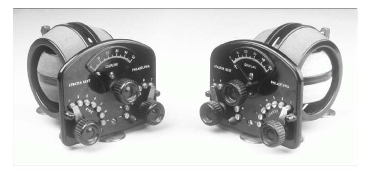
Figure 4-4. Mounted variocoupler # 3612 (black) or # 3734 (brown), left and right side views.
