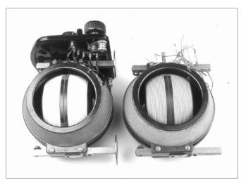
**Figure 4-8.** Left: mounted variocoupler # 3612 (black) or # 3731 (brown); Right: unmounted variocoupler # 3529 with string spacer in the rotor winding.
