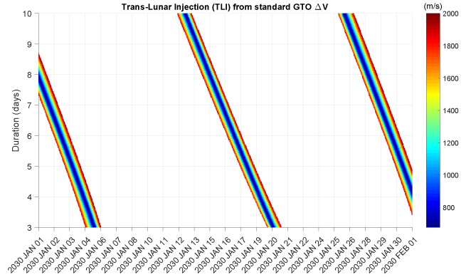
Fig. 17. TLI Delta-V from standard GTO in January 2030
