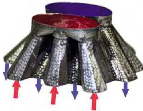
Figure 2. Heat exchanger produced with SLM. Source: See References
