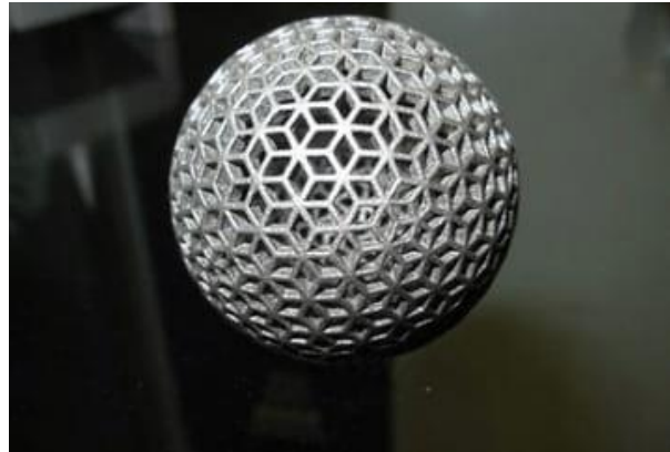
Figure 24. Metal part with a complex shape produced via SLM. Source: www.phoenixdeventures.com
