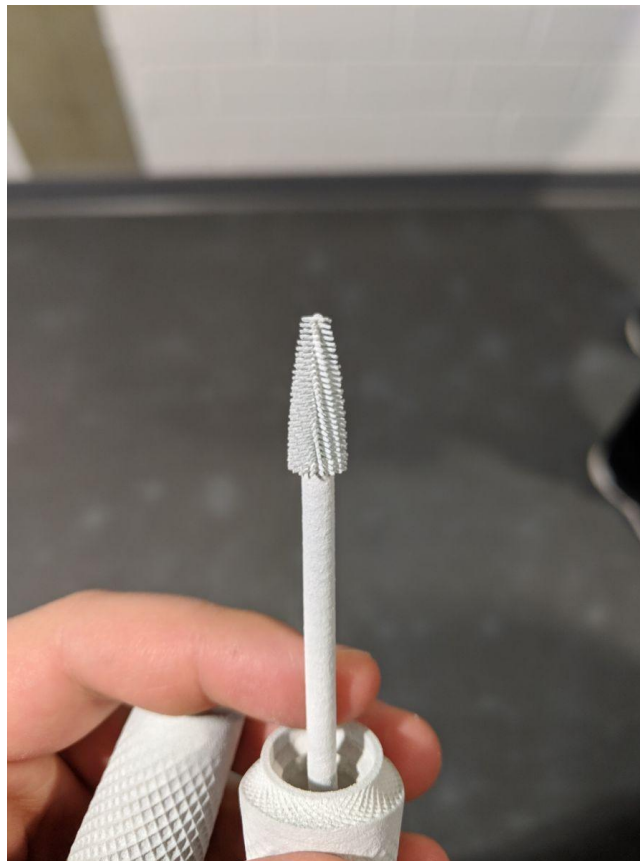
Figure 16. Example of SLS detail possibilities without supports. Source: L. Müller/Hochschule Düsseldorf.
