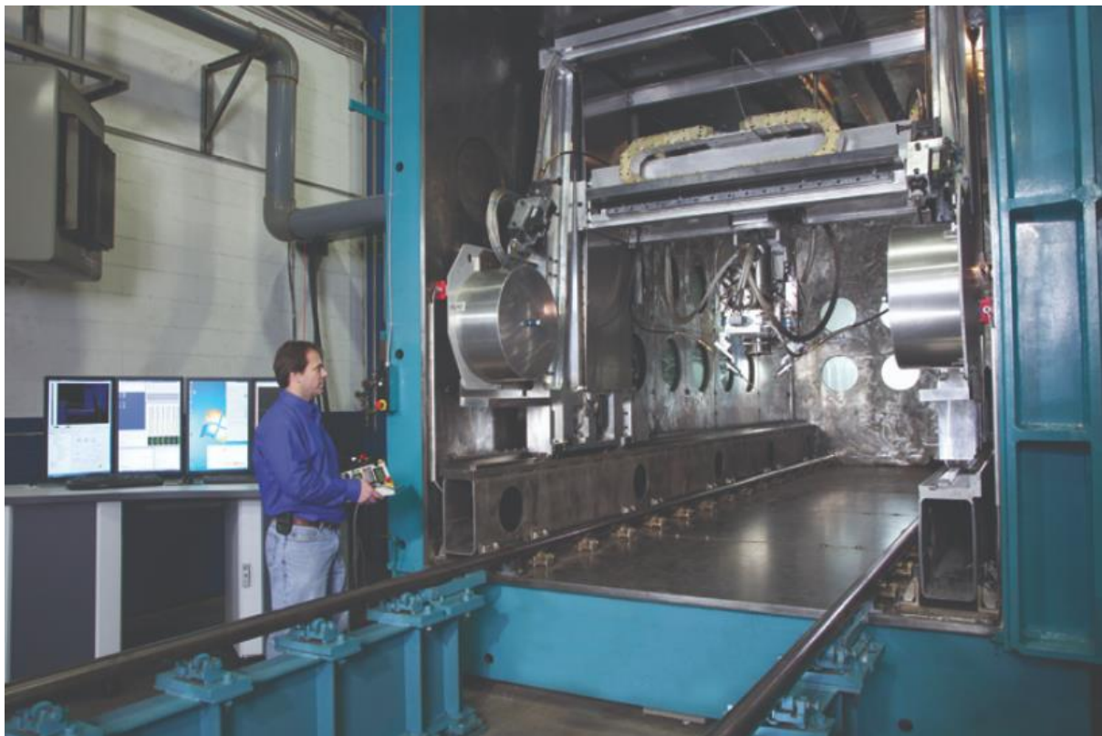
Figure 3. Sciaky EBAM 300 System. Source: www.sciaky.com
