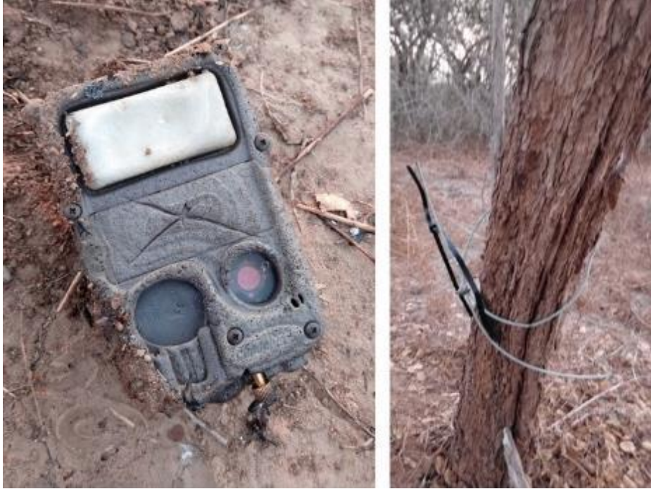
FIGURE 111 - LEFT: BURNED CAMERA TRAP; RIGHT: STOLEN CAMERA TRAP (STEEL CABLE LEFT BROKEN)
