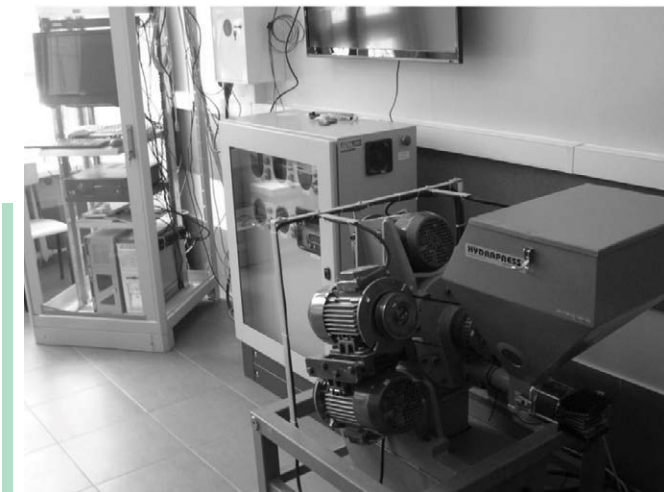
Rys. 3. The laboratory research stand of multidisc grinder
