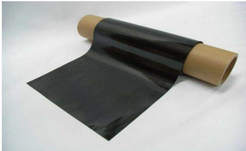
Figura 9 Pre-impregnat UD epòxid-carboni
