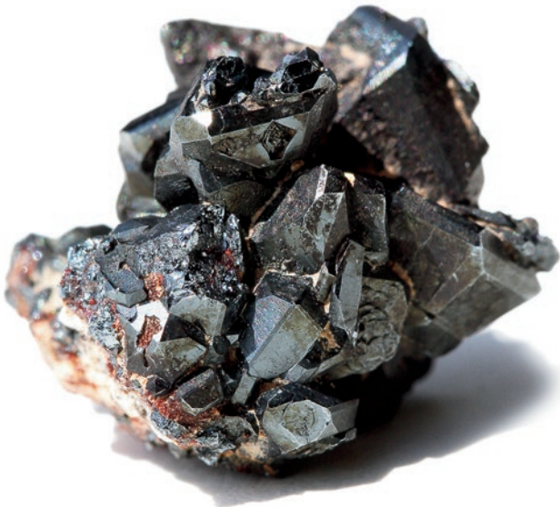
Figure 5. View of a large crystalline sample from Hisarcik. The large gray crystals are iron oxides (hematite) hosted on andesite visible in the lower left of the image. Tin oxide (cassiterite) is interspersed within and around the hematite and is visible as a bright red mineral here.
