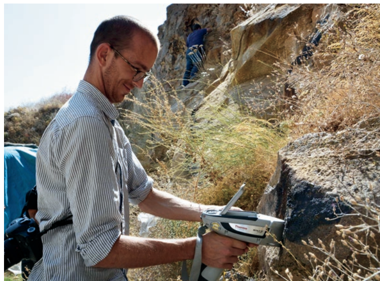
Figure 7. Taking in situ measurements of outcroppings at Hisarcık using a portable XRF. Photo courtesy of Gonca Dardeniz.
