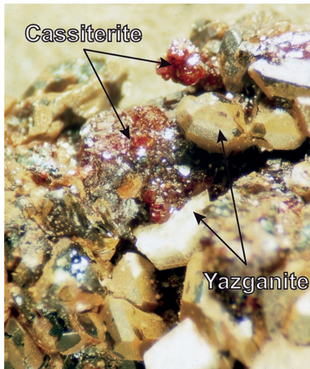
Figure 6. Microphotograph of cassiterite and yazganite minerals on a different sample of Hisarcık ore. Photo courtesy of Evren Yazgan.
