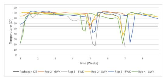
Figure 4. Temperature profiles of material in GORE<sup>®</sup> cells of composting cycle repetitions over time.
