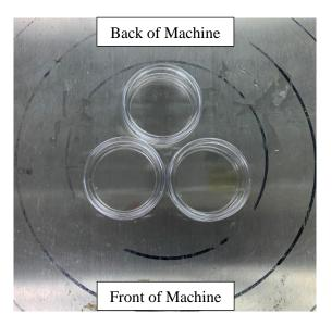
**Figure 1**. Plate orientation in Kimtron IC 350 X-ray machine.
