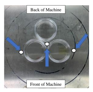
**Figure 2**. Representation of placement of dosimeters in Kimtron IC 350 X-ray machine.
