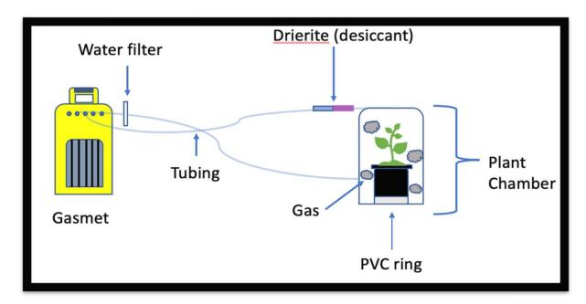
Figure 2. Depiction of gas sampling setup which includes (from left to right) Fourier transform infrared gas analyzer FTIR), 1/4" (6.35 mm) tubing creating a closed loop with a 6-gal (22.7-L) sealed chamber containing #2 containerized *Forsythia* placed upon a 1" (25.4 mm) PVC ring. A desiccant and water filter were added to the chamber return or FTIR intake to control humidity and protect internal mirrors.
