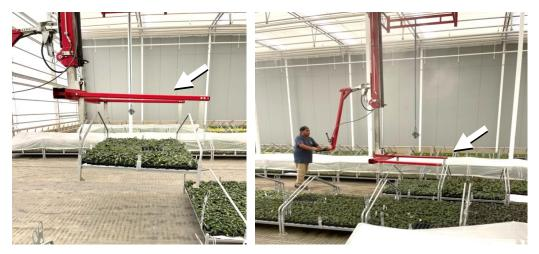
**Figure 3**. (Left) Flying forks (arrows) moving grow racks. (Right) Operator controlling grow racks.
