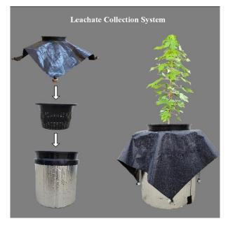
**Figure 2**. Illustration of the leachate collection system.
