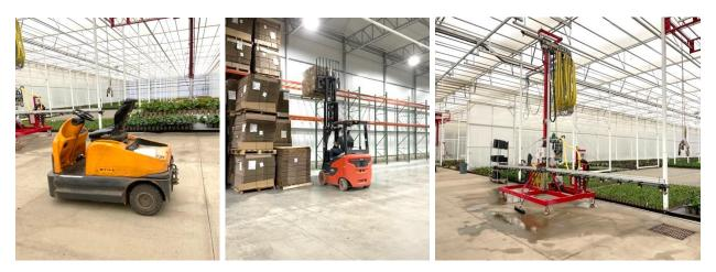
Figure 2. (Left) Battery powered tugger, (center) forklift, and (right) and electric boom.
