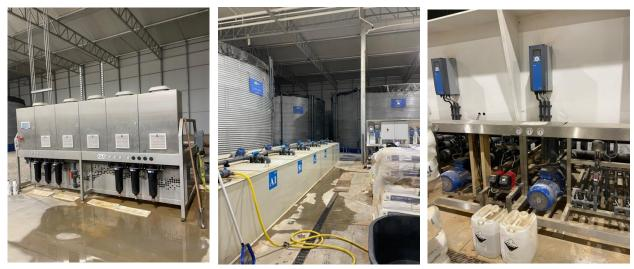
**Figure 5**. (Left) Fog machine, (center) fresh water tank, and fertilizer recipe tanks for flood-floor, and (right) fertilizer injectors.
