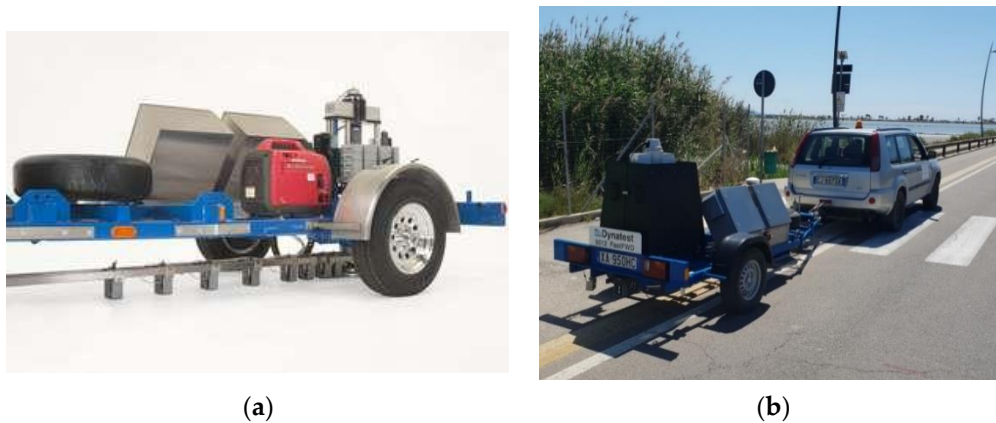
Figure 1. (a) Fast Falling Weight Deflectometer (Fast-FWD) with the main elements: falling mass and geophones of measure bar [37] and (b) on trailer towed by vehicle ready for testing.
