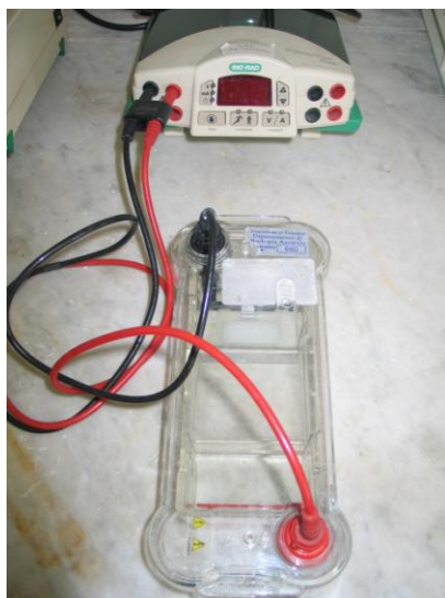
Fig. 14: “Mini-Protean II electrophoresis Cell” e “Sub-Cell GT Agarose Gel Electrophoresis Systems”
