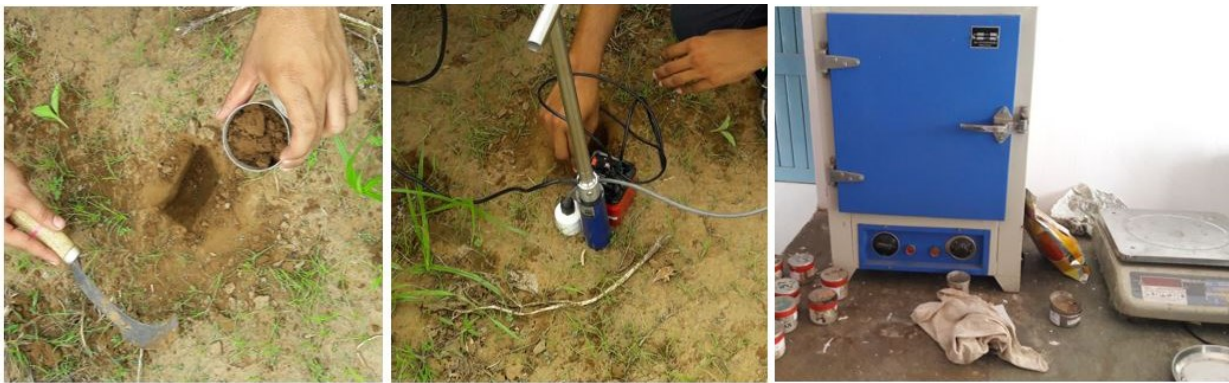
Figure 3: (a) Soil sampling at 5 cm, (b) Placement of sensors around sampling site and (c) Oven drying samples
