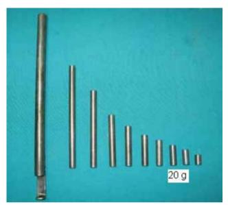
**Fig. 1.** The trauma set prepared for the study: a 30 cm metal tube with a spoon mechanism at its lower tip and cylinder-shaped metal weights of 100, 75, 50, 40, 30, 25, 20, 15, 10 g, respectively. *(Color figure can be viewed in the online issue, which is available at www.tjtes.org)*
