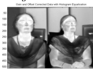
Figure.8. Gain and Offset corrected data with Histogram Equalization
